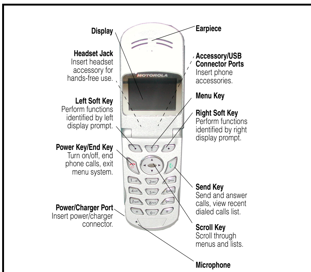
Figure 1. Telephone Controls, Indicators, and I/O
