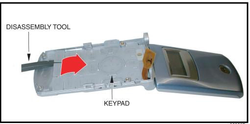
Figure 12. Removing the Keypad
