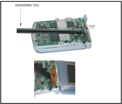
Figure 11. Disconnecting the Flex From the Transceiver Board
