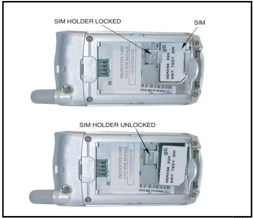
Figure 6. Removing the SIM
