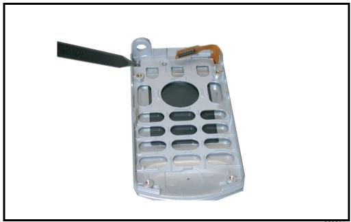
Figure 14. Removing the LED Light Guard
