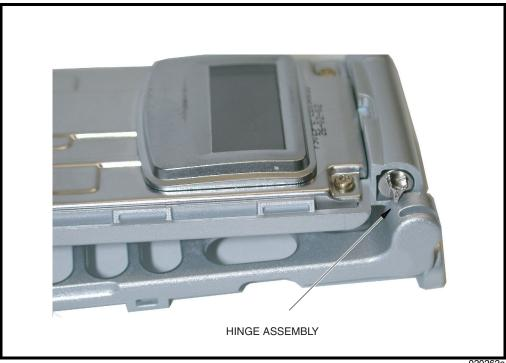
Figure 17. Replacing the Hinge Assembly
