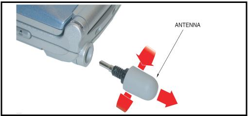
Figure 7. Removing the Antenna
