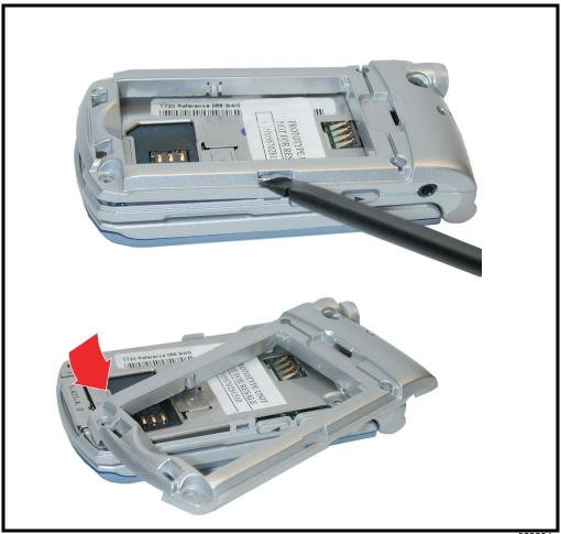
Figure 9. Removing the rear housing assembly
