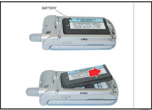
4. Lift the end of the battery and remove it completely (See Figure 5).
