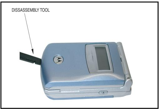
Figure 13. Removing the Flip Cover
