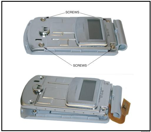
Figure 18. Removing the Display Module
