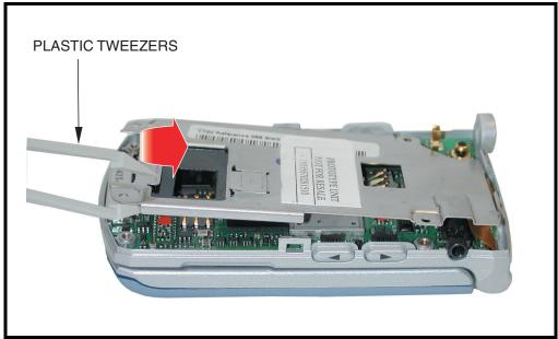
Figure 10. Removing the Chassis Shield
