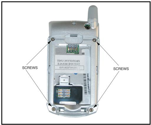
Figure 8. Removing the Rear Housing Assembly Screws
