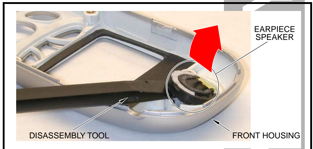
Figure 17. Removing the earpiece speaker
