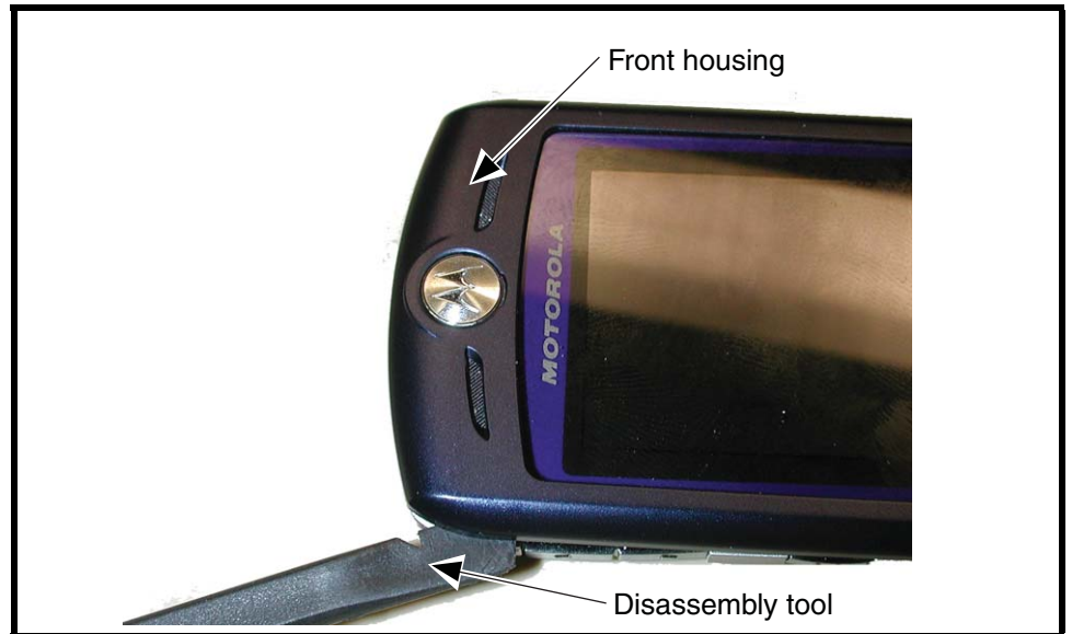
Figure 14. Releasing the Front Housing Catches
