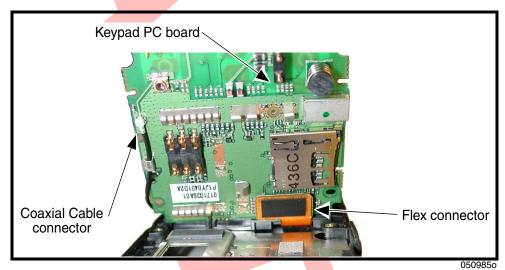
Figure 18. Removing the Keypad PC Board Flex Connector
