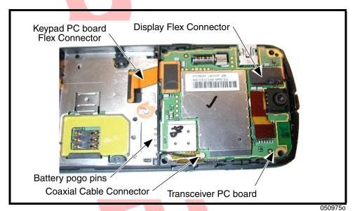
Figure 10. Removing the Transceiver PC Board Connectors
