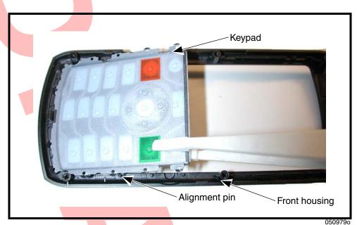
Figure 16. Removing and Replacing the Keypad
