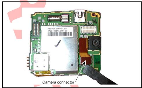
Figure 13. Removing the Camera Assembly
