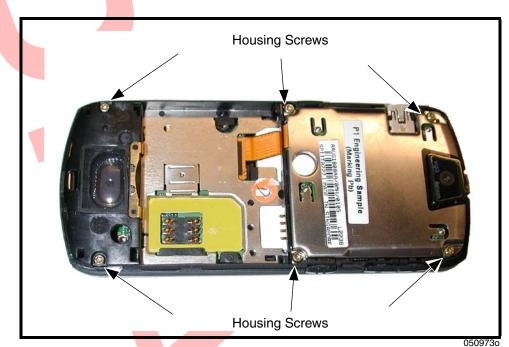
Figure 8. Removing and Replacing the Transceiver PC Board Shield.
