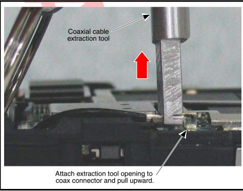
Figure 12. Coaxial Cable Extraction Tool
