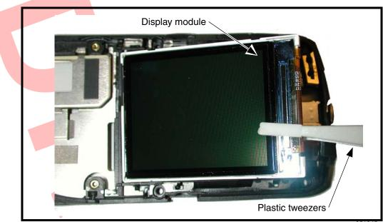
3. Turn the chassis assembly over and lift the top edge of the display module (see Figure 21).
