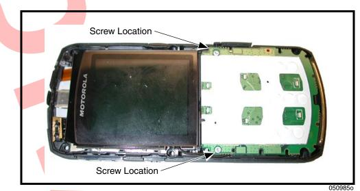
Figure 17. Removing the Keypad PC Board Screws
