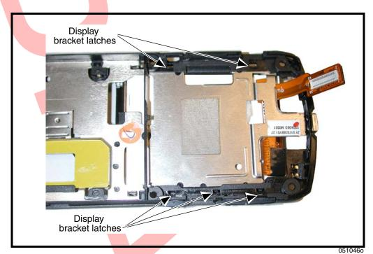
Figure 20. Removing the Display Module Latches
