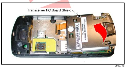
Figure 9. Removing and Replacing the Transceiver PC Board Shield.
