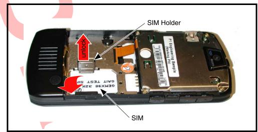
Figure 6. Removing and Replacing the SIM
