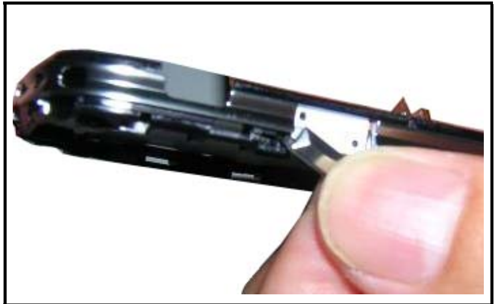
Figure 15. Removing the Side Key
