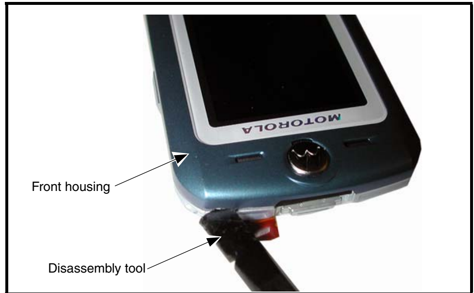
Figure 25. Releasing the Front Housing Catches
