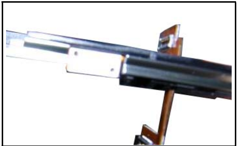
Figure 21. Adhering the flex onto the Chassis Side Wall
