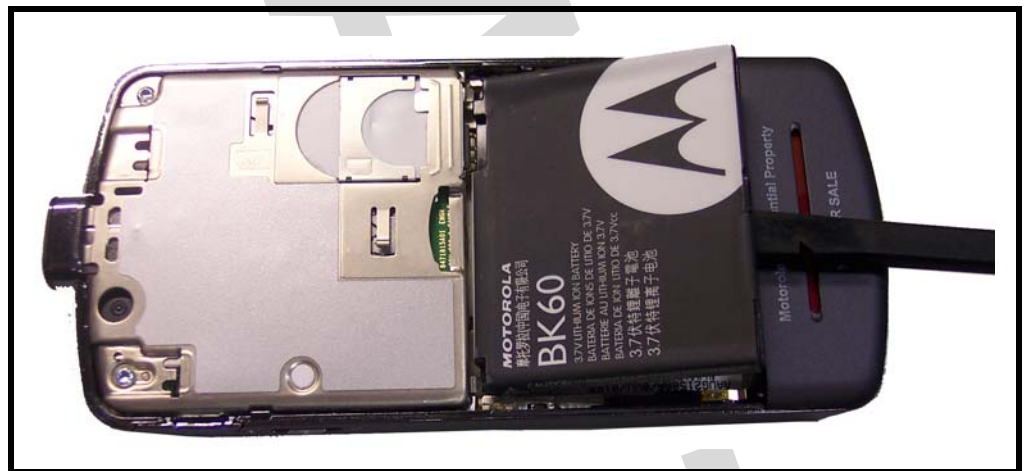
Figure 3. Removing the Battery
