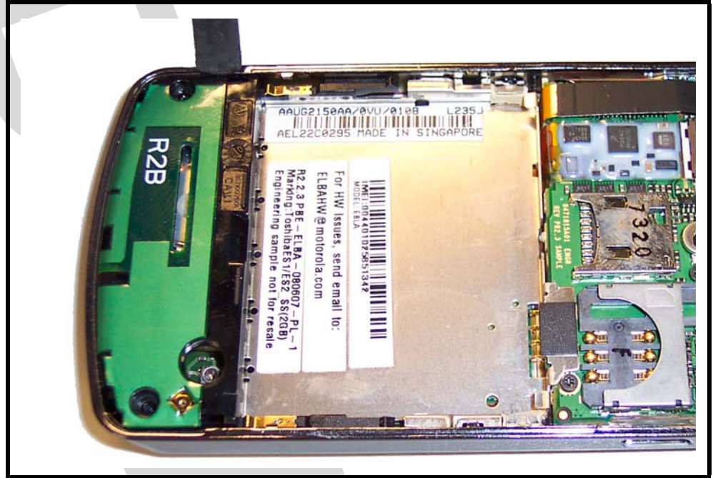
Figure 9. Removing the Acoustic Chamber Assembly
