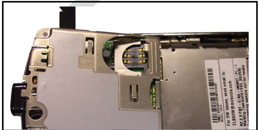
Figure 7. Removing the PCB Cover
