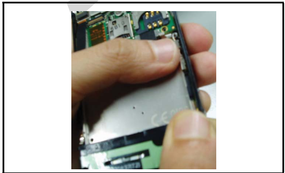
Figure 11. Aligning the Acoustic Chamber Assembly
