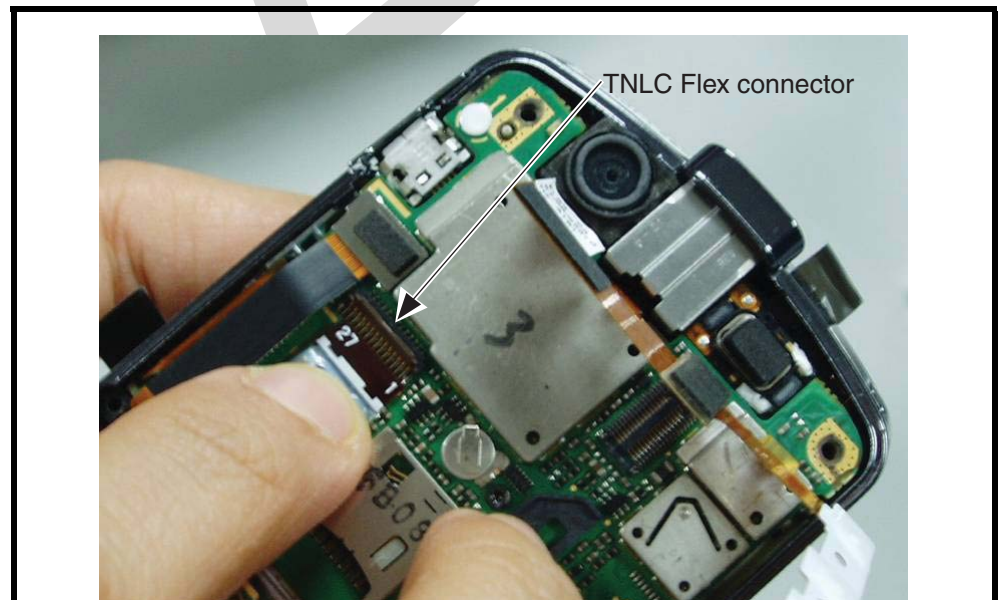
Figure 36. Connecting TNLC Flex to the Transceiver PCB
