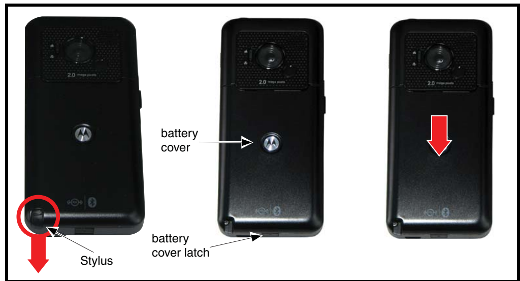
Figure 1. Removing the Battery Door
