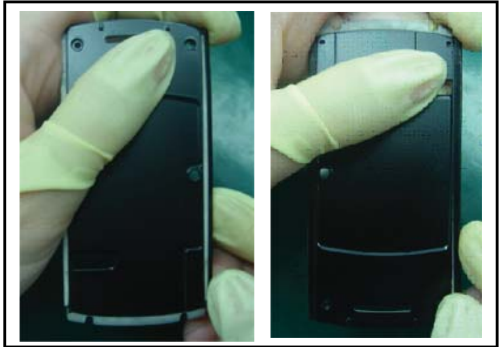
Figure 49. Rail Assembly on Slider Inner Assembly
