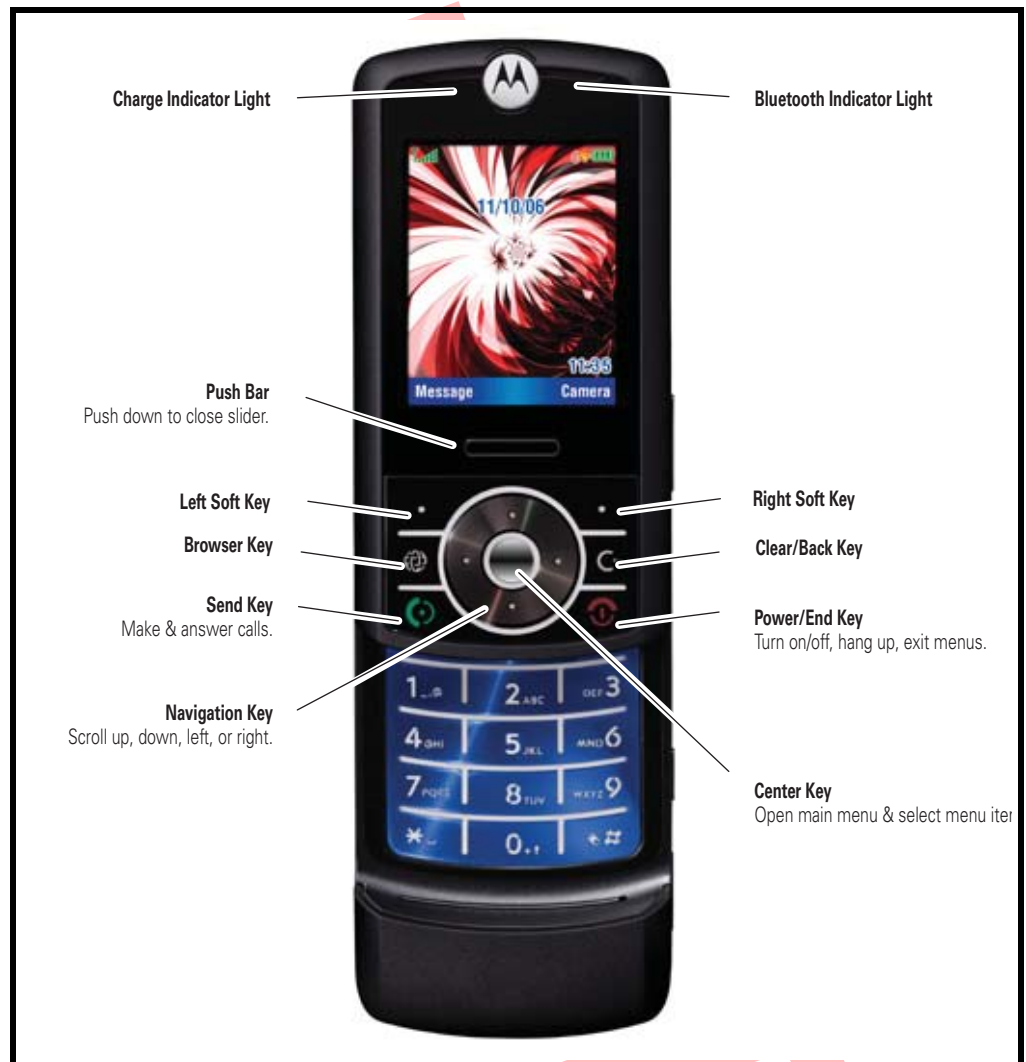
Figure 1. Controls, indicators, and I/O
