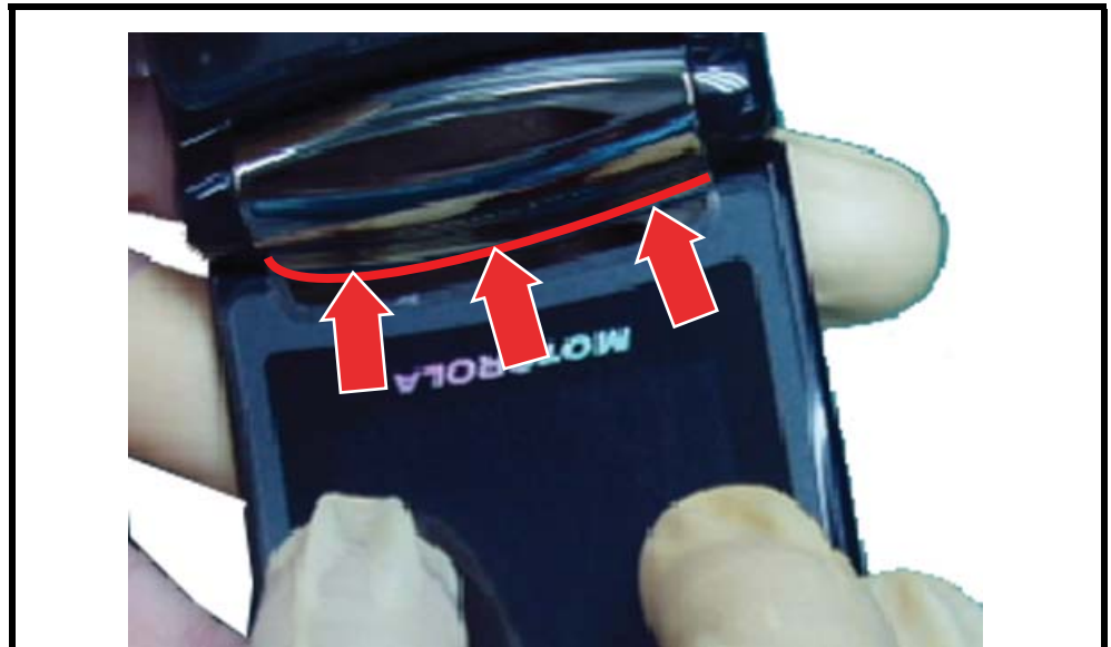
Figure 72. Attaching the Main Lens
