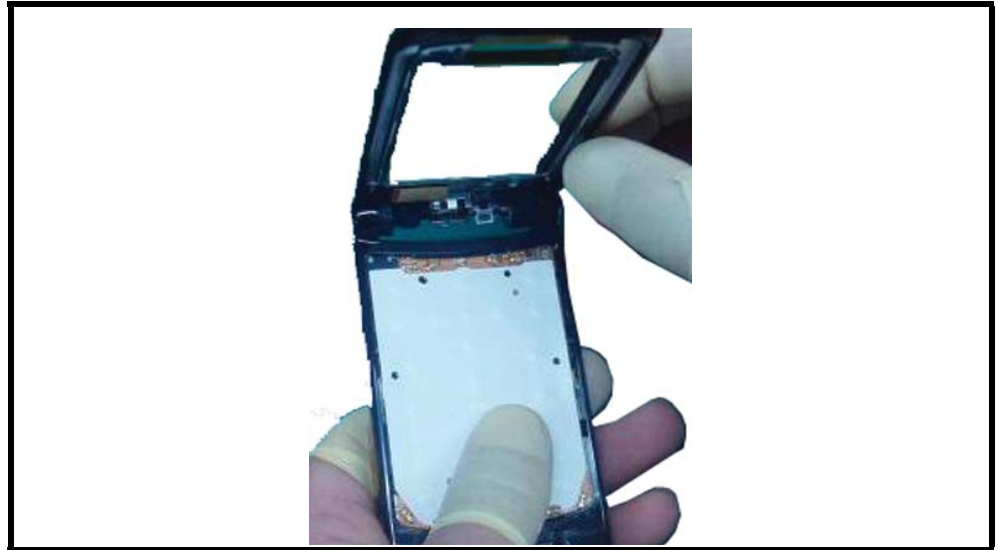
Figure 52. Inspecting the Flip Assembly
