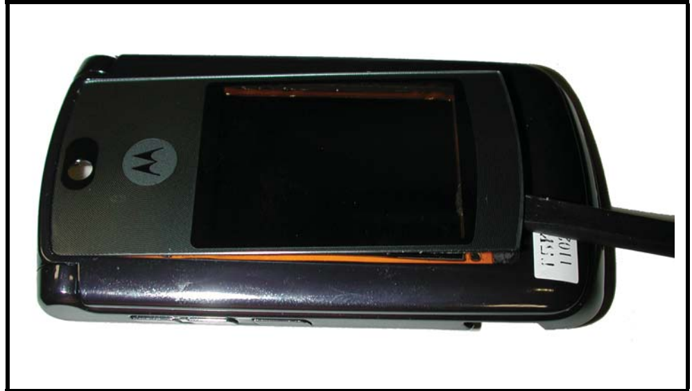
Figure 25. Prying the CLI Lens
