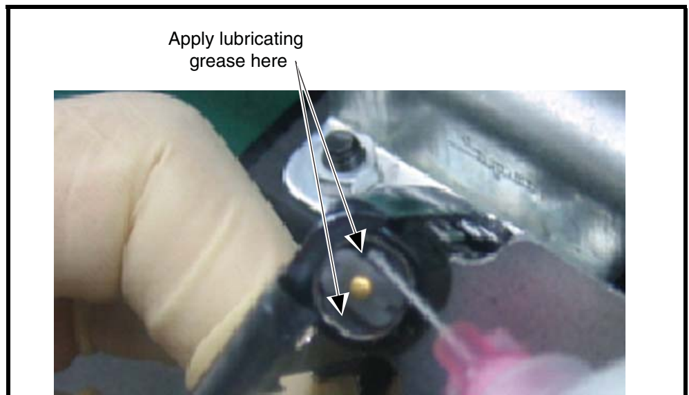
Figure 49. Lubricating the Flip Hinge
