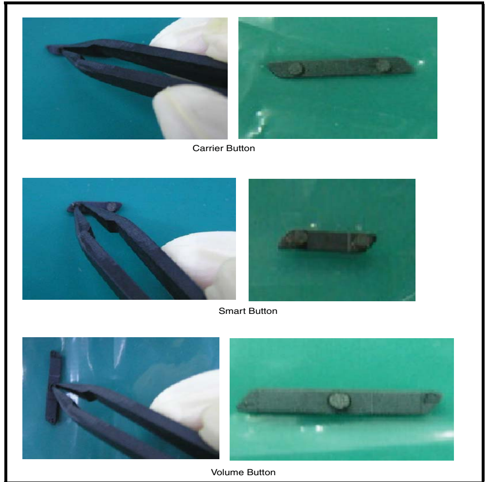
Figure 45. Installing the Side Key Pads
