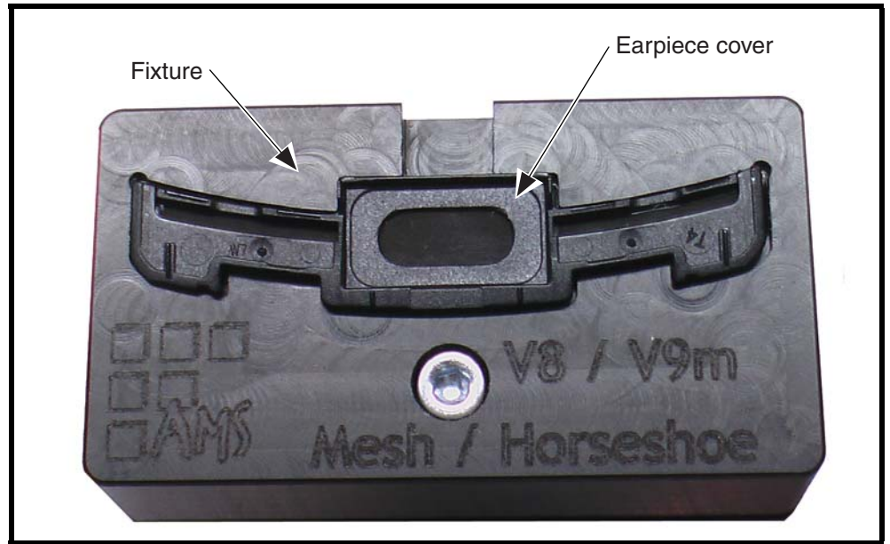
Figure 62. Earpiece Cover in the Fixture
