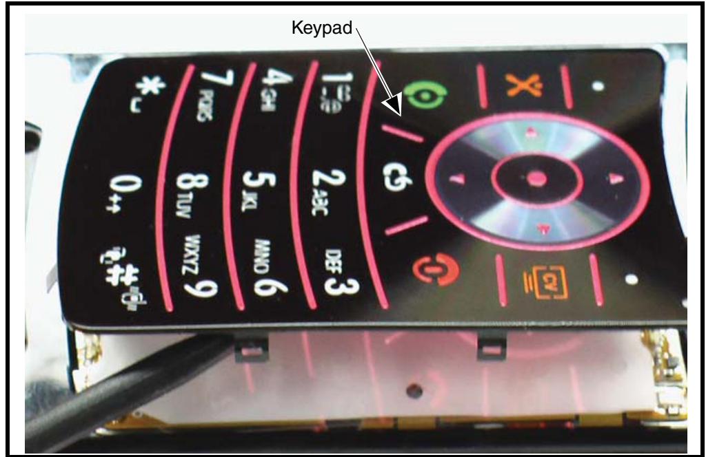
Figure 20. Placing the Keypad into the Front Housing
