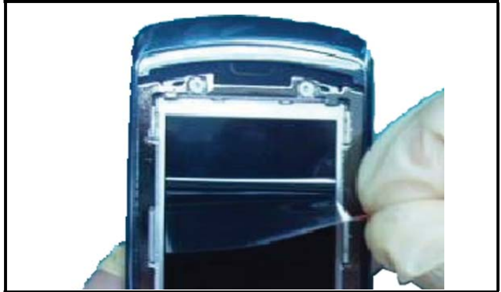
Figure 71. Removing the LCD Liner
