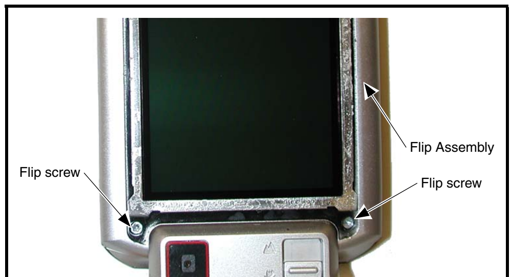
Figure 18. Removing the Bottom Flip Screws
