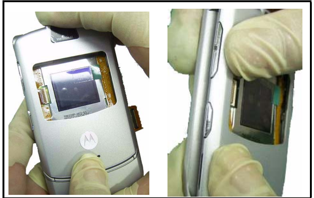
Figure 16. Flip Cover Replacement
