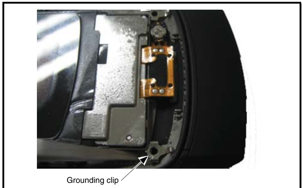
Figure 21. Removing the Grounding Clips
