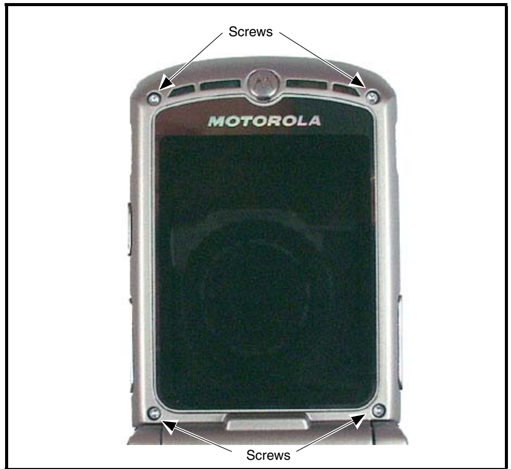
Figure 10. Removing the Flip Assembly Screws
