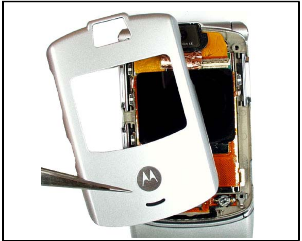
Figure 12. Removing the Flip Assembly Cover
