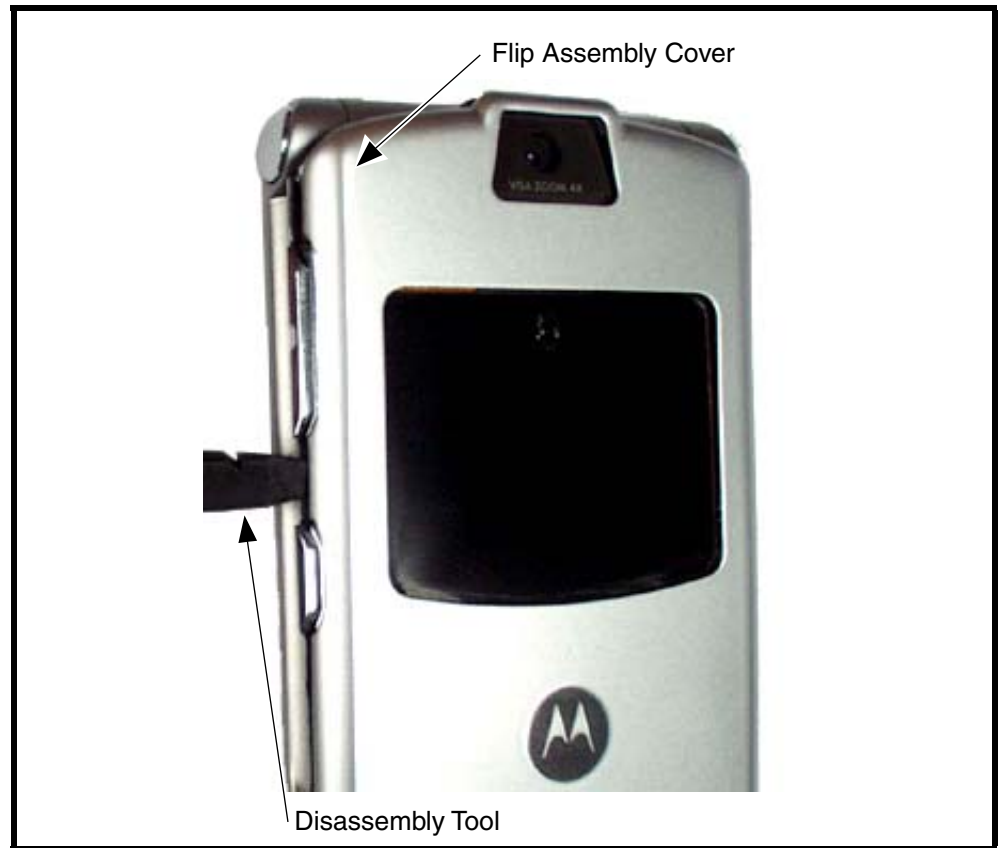
Figure 11. Separating the Flip Assembly Cover
