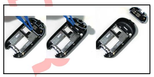
Figure 19. Removing the Antenna from the Housing
