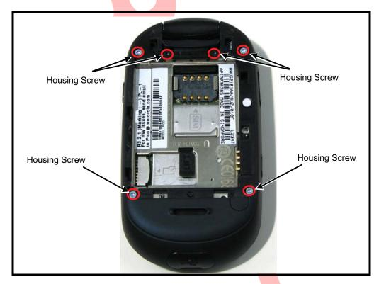
Figure 4. Removing the Rear Housing Screws
