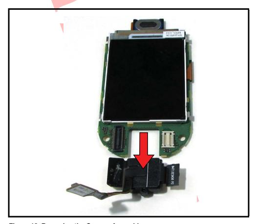
Figure 18. Removing the Camera Assembly
