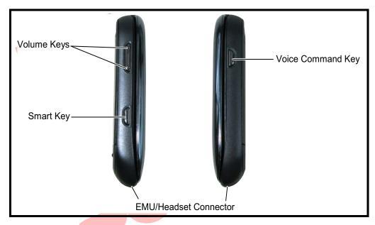
Figure 3. Telephone Controls and Indicators Locations (Sides)
