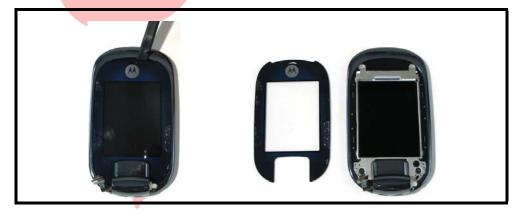
Figure 10. Removing the Main Lens to Expose Housing Screws
