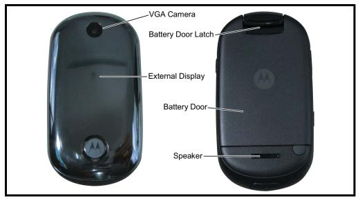
Figure 2. Telephone Controls, indicators, and I/O Connections (Flip Closed)
