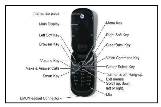
Figure 1. Telephone Controls, indicators, and I/O Connections (Flip Open)
