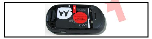
Figure 2. Removing the Battery
