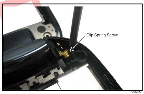
Figure 7. Clip Spring Removal
