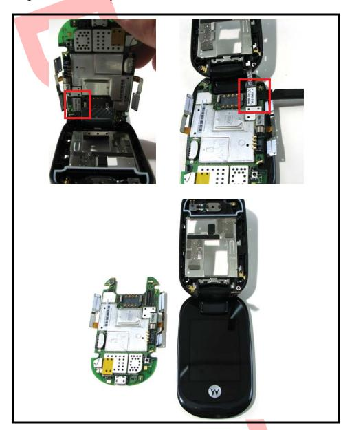
Figure 6. Locating and Separating the Main Flex Connector
