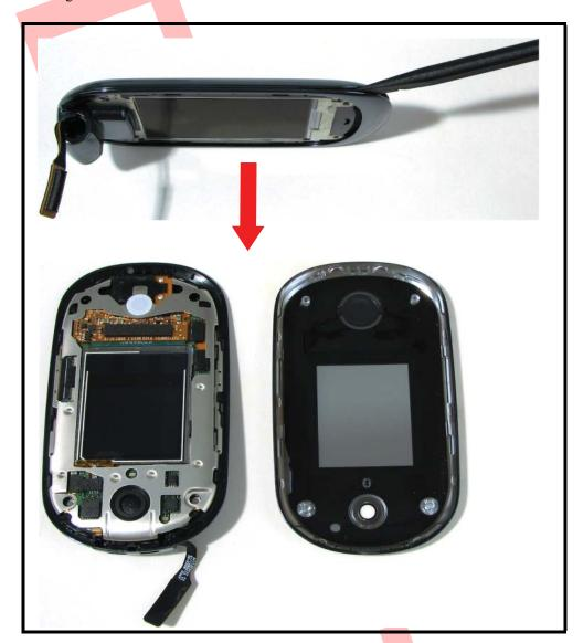
Figure 12. Separating the Flip Front Housing from the Flip Rear Housing
