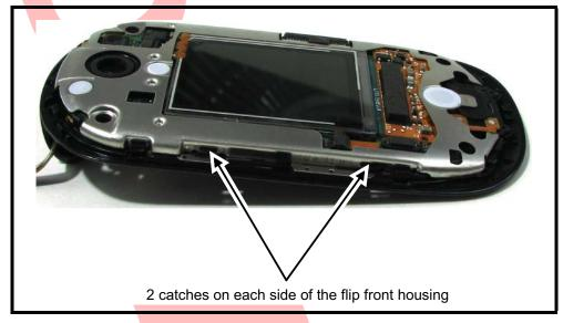
Figure 14. Disengaging the Display Bracket Assembly Catches
