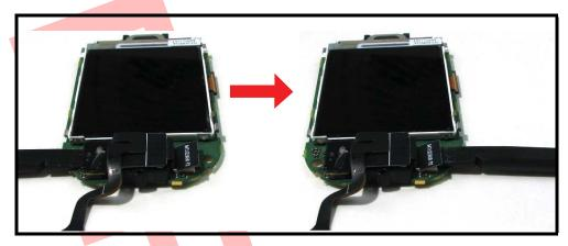
Figure 17. Unseating the Camera and Flip Flex Connectors
