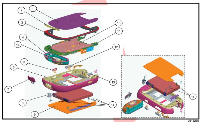
Figure 22. Exploded View Diagram (Flip Assembly)
