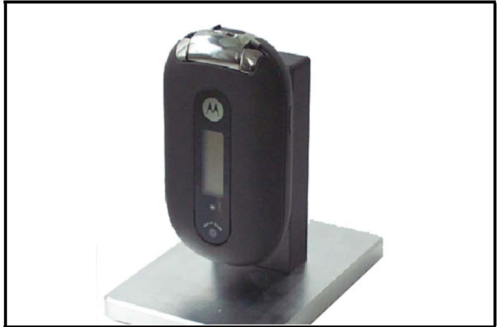
Figure 13. Insert the U6 Onto the Test Fixture
