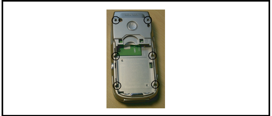
Figure 17. Removing the 6 Screws from the Rear Housing Cover
