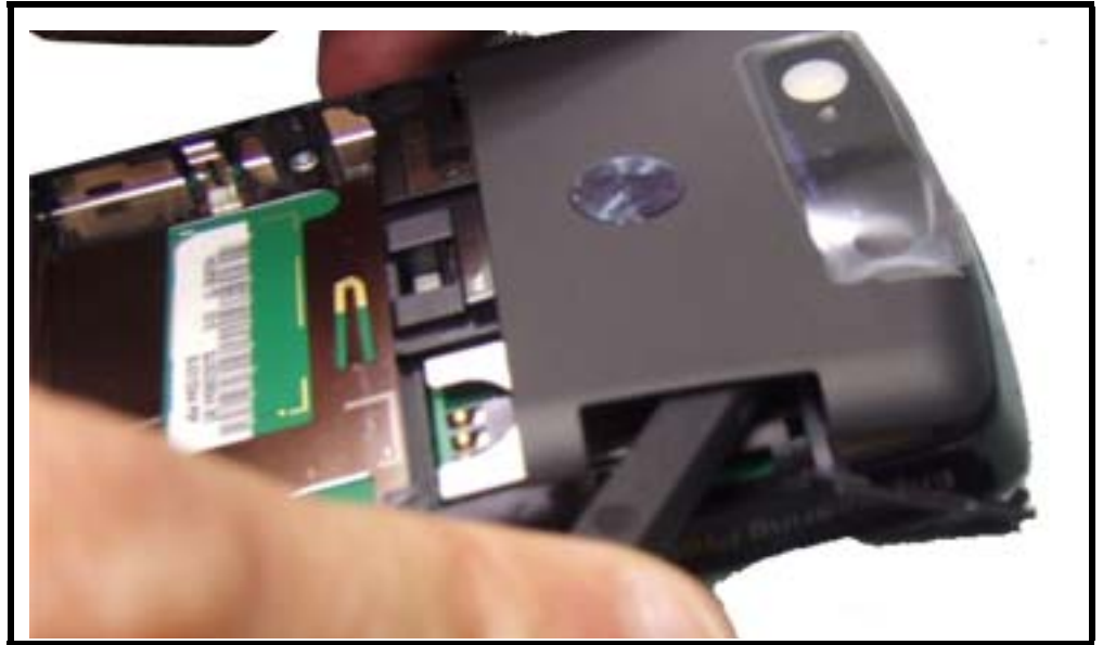
Figure 9. Removing the Rear Top Cover
