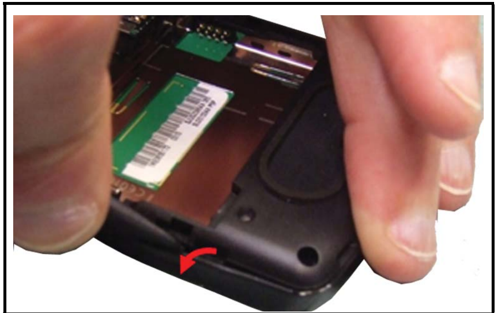
Figure 14. Removing the Rear Housing Snaps
