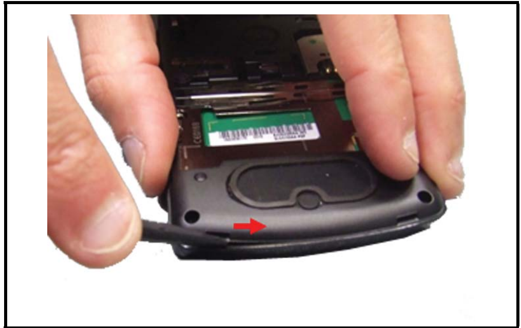
Figure 15. Removing the Rear Housing Snaps
