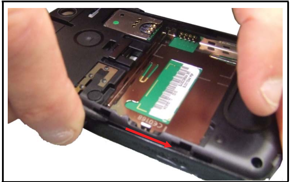
Figure 13. Removing the Rear Housing Snaps
