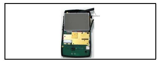
Figure 26. Removing the Display Module
