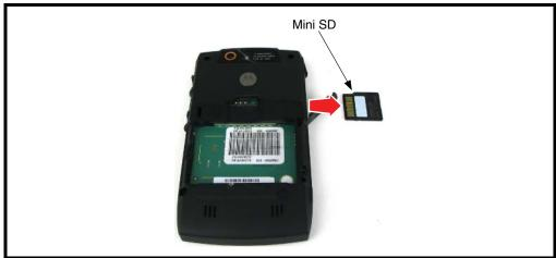
Figure 4. Removing the Memory Card
