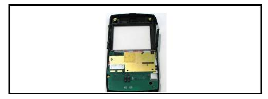
Figure 27. Display Module Removed
