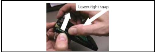
Figure 8. Disengaging the Lower Right Snap
