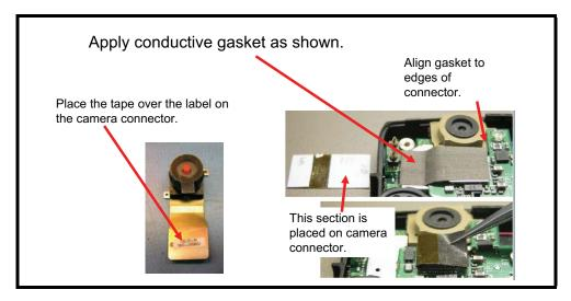
Figure 16. Camera Assembly Placement
