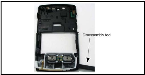
Figure 24. Removing the Antenna
