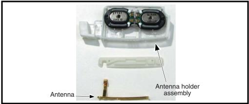
Figure 25. Separating the Antenna Assembly
