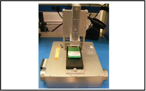
Figure 23. Removing the Display Connector Pad
