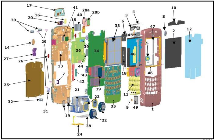
Figure 33. Exploded View Diagram (Main assembly)
