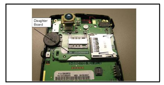
Figure 14. Camera Assembly Removal
