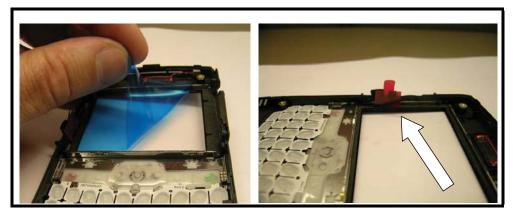
Figure 28. Removing the Protective Liners
