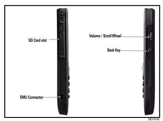
Figure 2. Telephone Controls and Indicators Locations (Sides)
