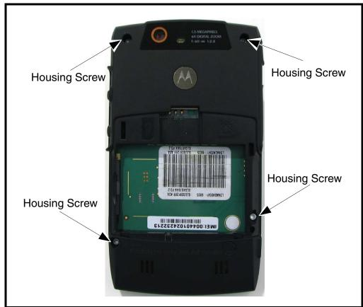
Figure 5. Removing the Rear Speaker Housing Screws
