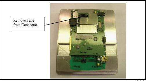
Figure 22. Removing the Display Connector Pad
