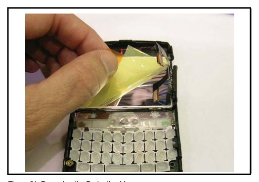
Figure 31. Removing the Protective Liner
