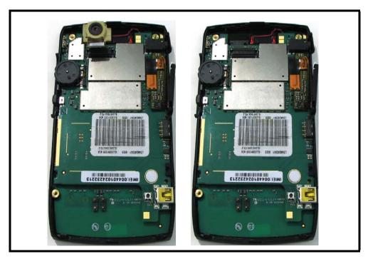
Figure 12. Camera Assembly Removal
