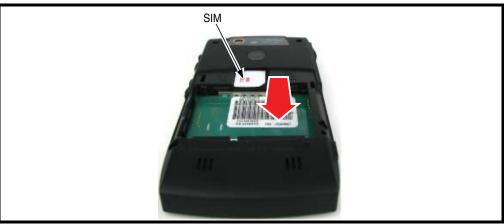
Figure 3. Removing the SIM
