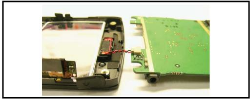
Figure 19. Separating the Main Board from the Front Housing
