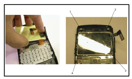
Figure 30. Inserting the Display Module
