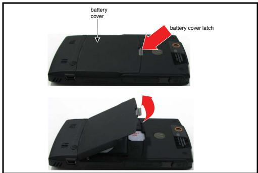
Figure 1. Removing the Battery Door
