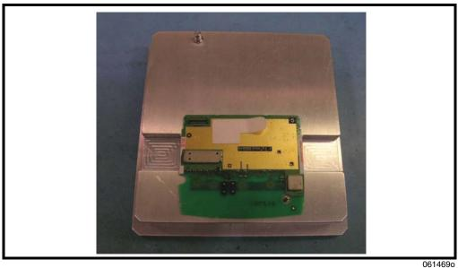
Figure 21. Removing the Display Connector Pad
