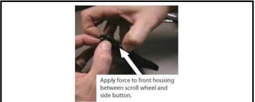
Figure 7. Removing the Scroll Wheel
