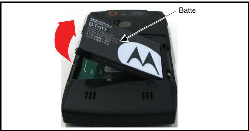
4. Lift the end of the battery and remove it completely. See Figure 2.
