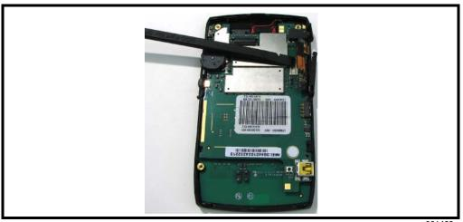
Figure 18. Disconnecting the Flex from the Display Module
