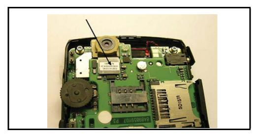
Figure 15. Camera Assembly Placement
