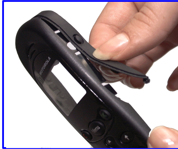
14. Remove flexible strip by holding the front housing facing downwards and pulling strip up
