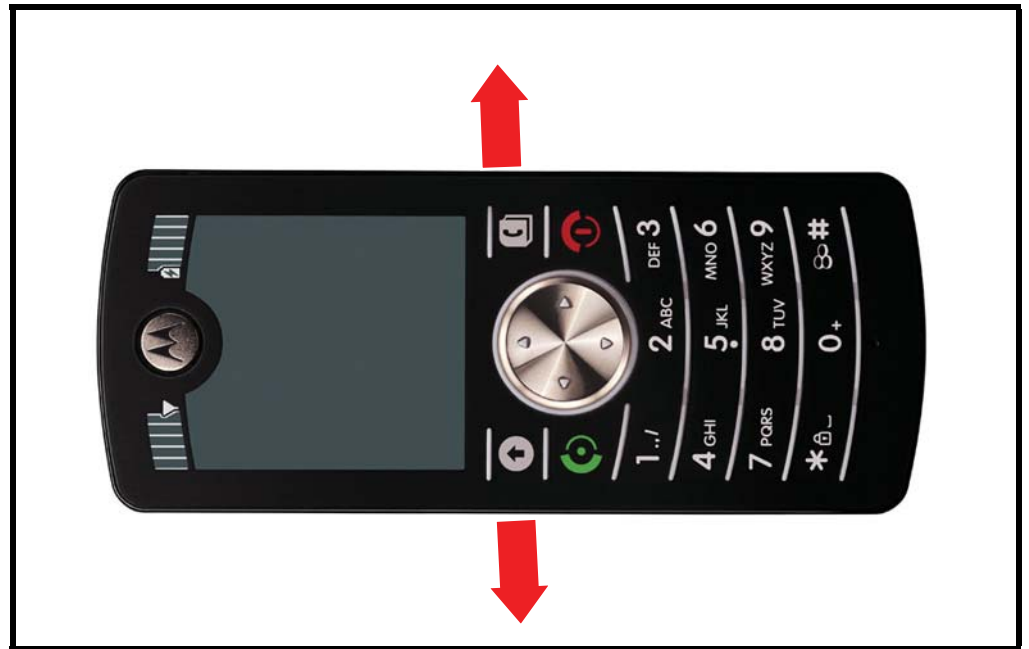
Figure 8. Releasing the Side Housing Latches
