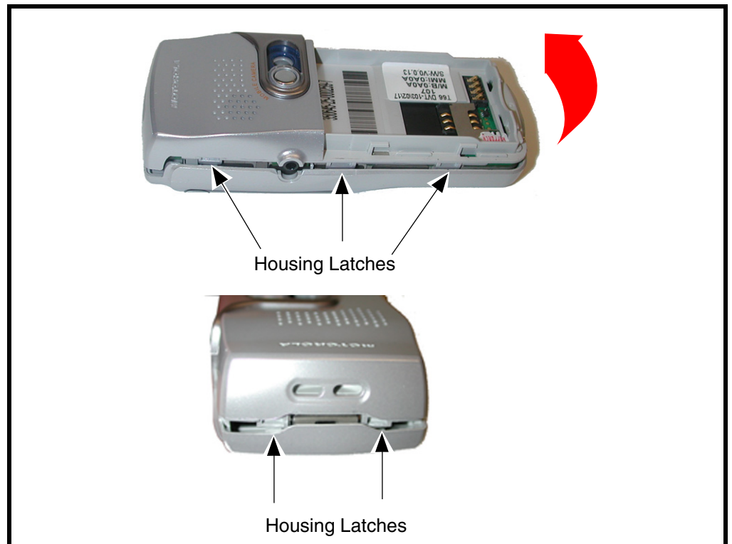
Figure 4. Removing the Front Housing Cover
