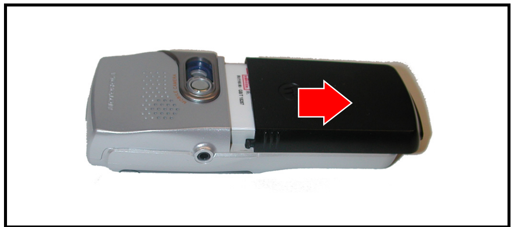
Figure 1. Removing the Battery Cover
