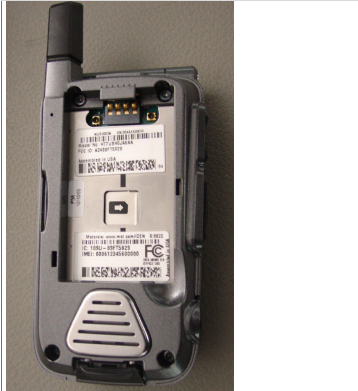
Photograph 3.6: Back view, battery cover removed.
