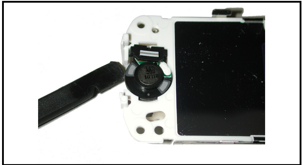
Figure 16. Removing the Front Speaker
