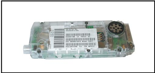
Figure 8. Removing and Replacing the Endo Housing
