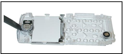
Figure 15. Removing the Front Speaker
