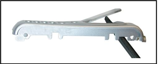
Figure 10. Removing and Replacing the Display Lens
