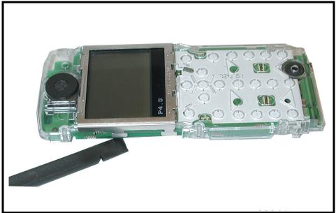
Figure 12. Removing the LCD Module Assembly
