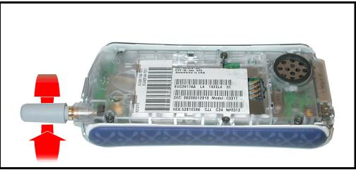
Figure 6. Removing the Antenna
