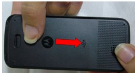
1. Push the latch to remove battery housing
