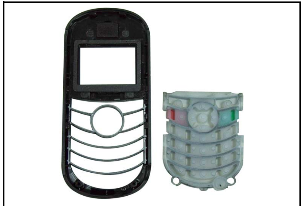
Figure 11. Removing the rubber keypad
