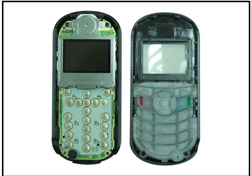
Figure 10. Removing the front housing
