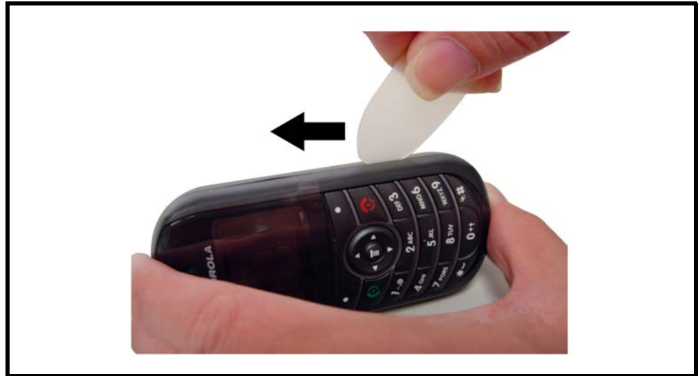
Figure 9. Prying the case apart along the seam
