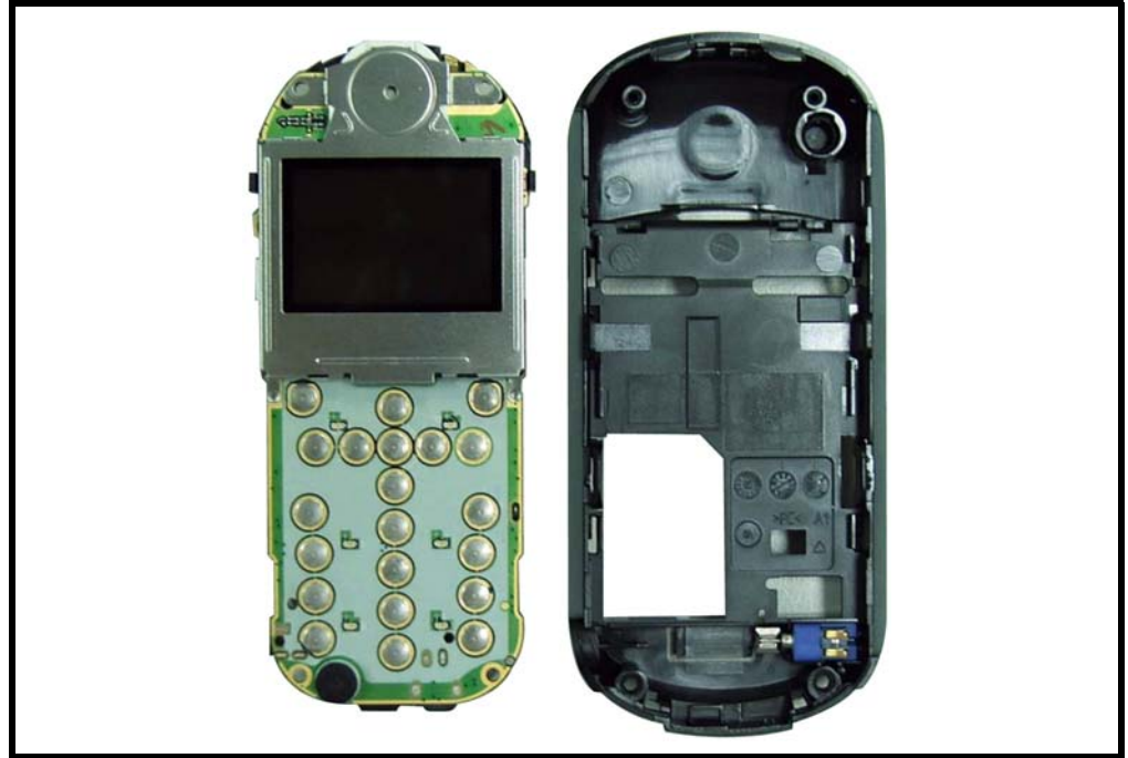
Figure 13. Disengaging the side latches
