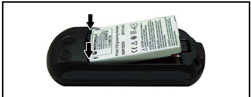
Figure 6. Replace the battery cover
