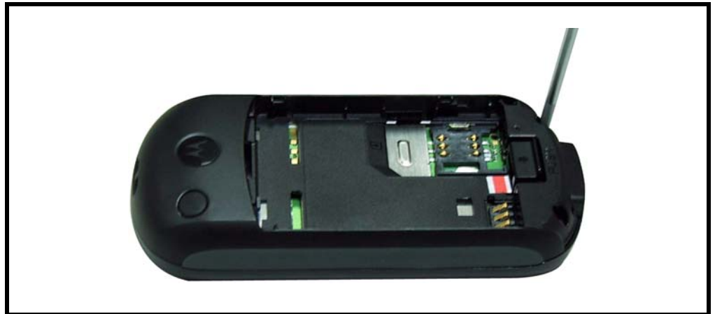
Figure 8. Removing the two T5 screws (T-force = 1.4 kgf-cm)
