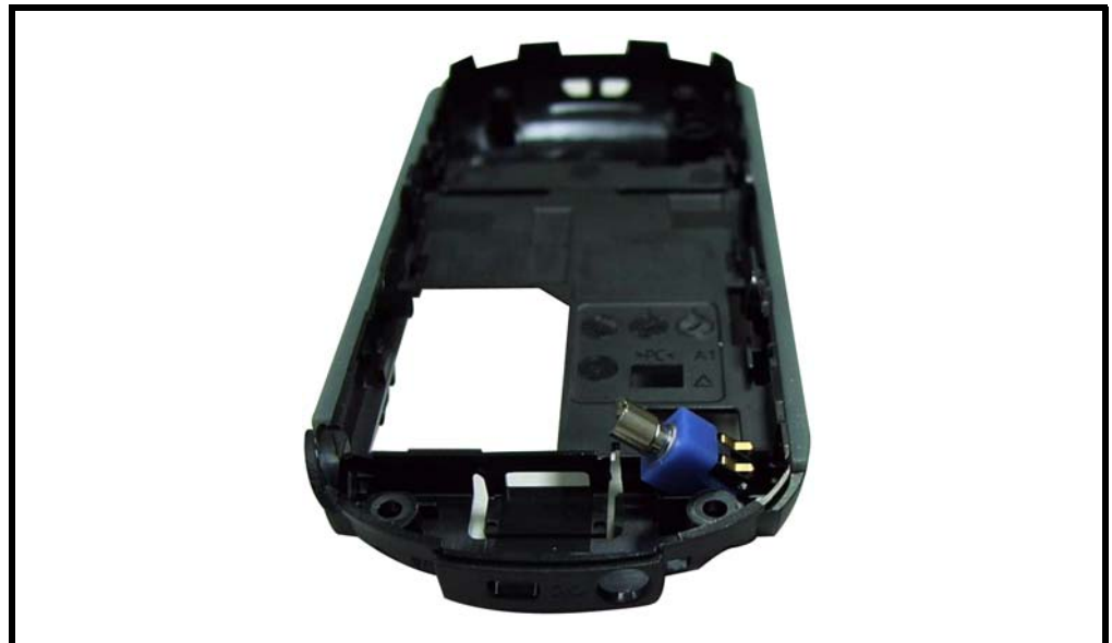
Figure 14. Removing the vibrator module
