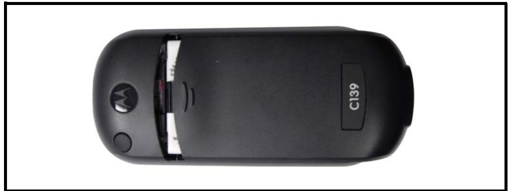
Figure 5. Removing the battery cover
