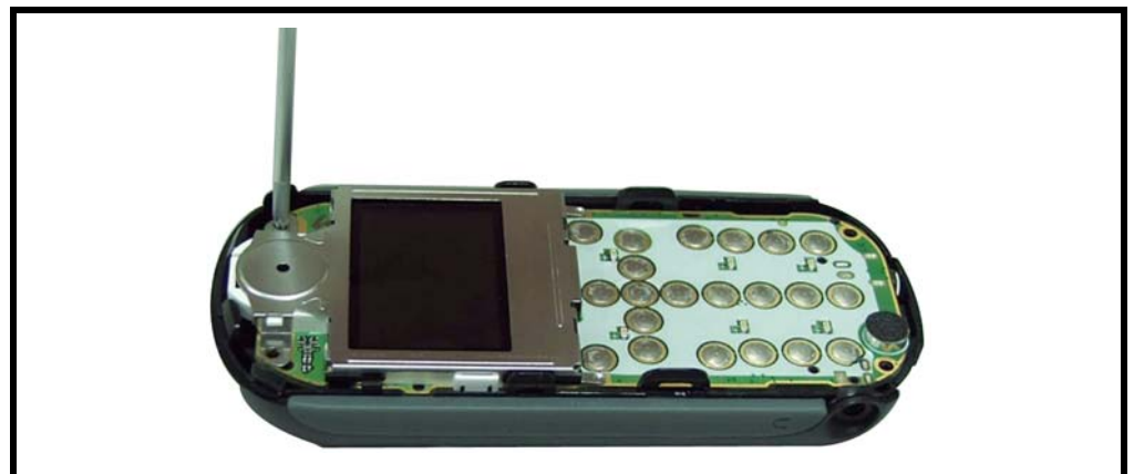
Figure 12. Removing two T5 screws (T-force = 1.4 kgf-cm)
