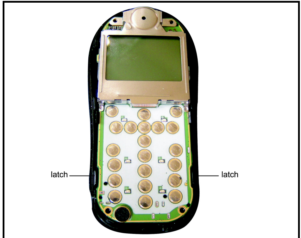
Figure 14. Pry open the side latches securing the Transceiver board to the back housing
