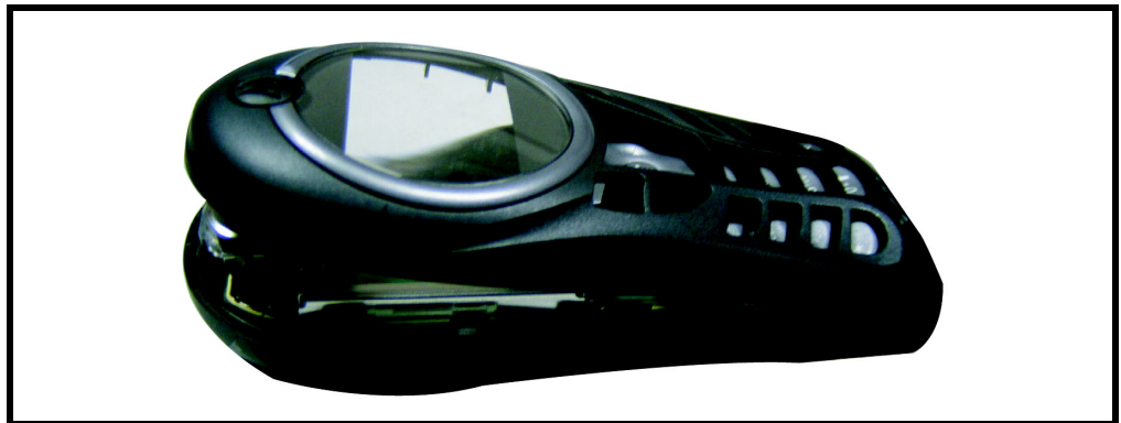
Figure 11. Remove the front housing
