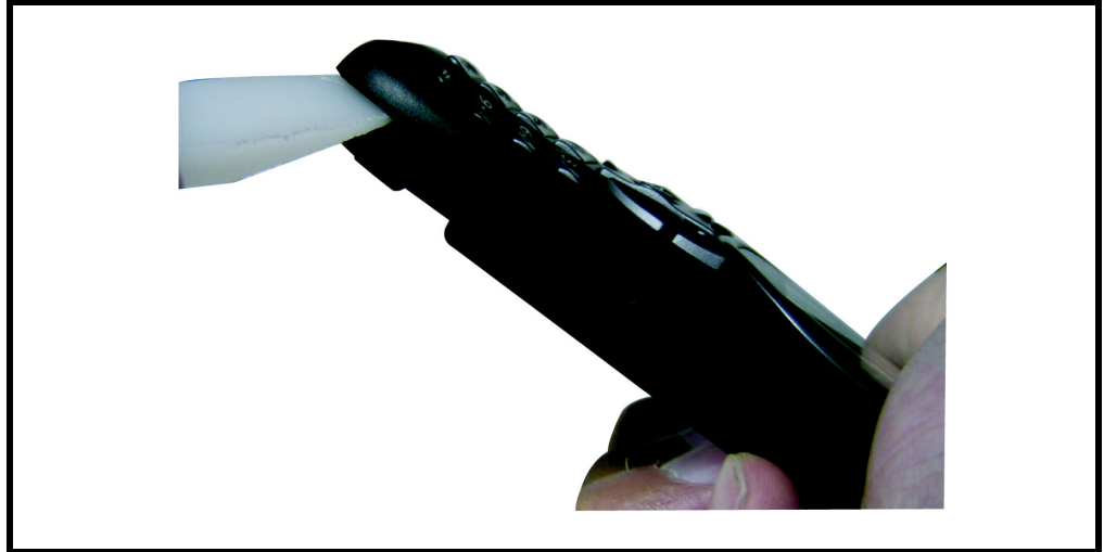
Figure 10. Use a flat wedge tool to pry the case
