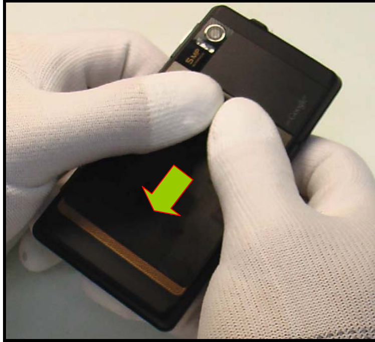
Figure 1. Releasing Battery Door
