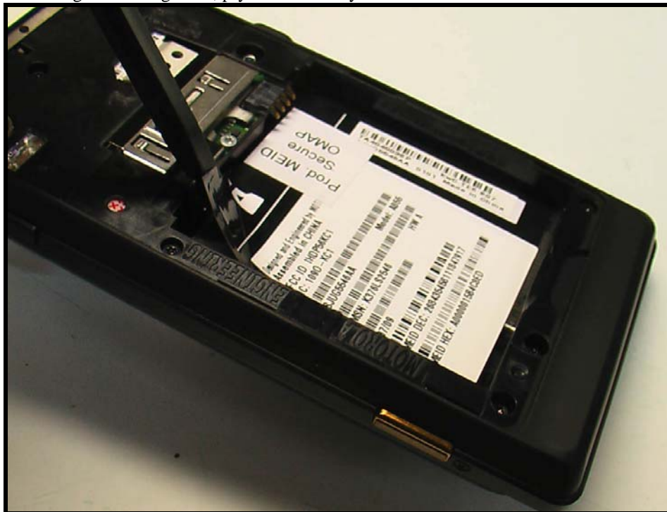
Figure 7. Removing the battery label
