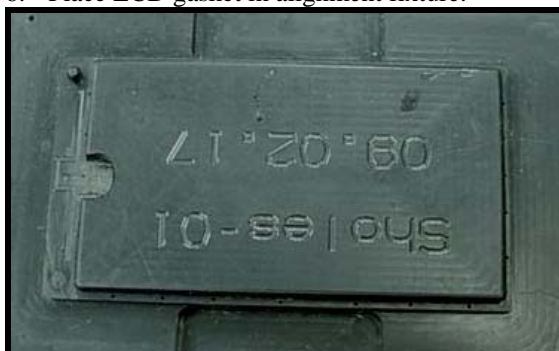
Figure 62. Aligning LCD gasket
