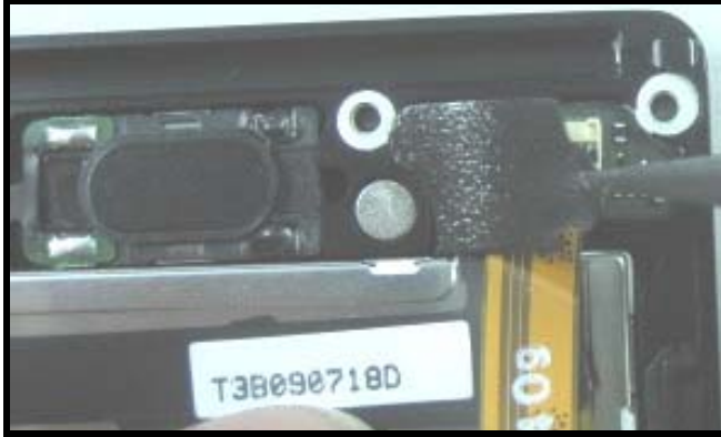
Figure 77. Placing water ingress over display connector
