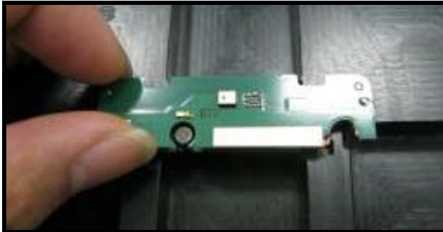
Figure 120. Audio board alignment
