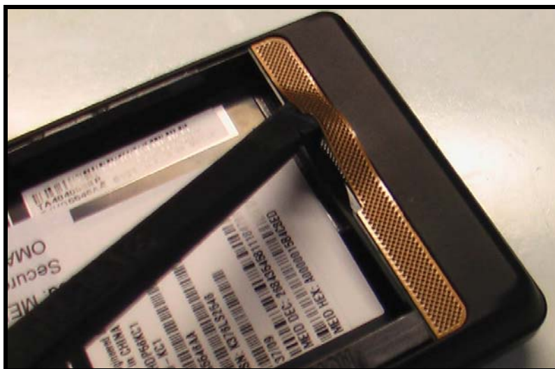
Figure 5. Removing the speaker grill
