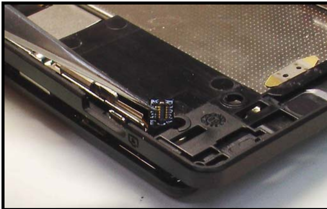
Figure 104. Lifting Side flex connector
