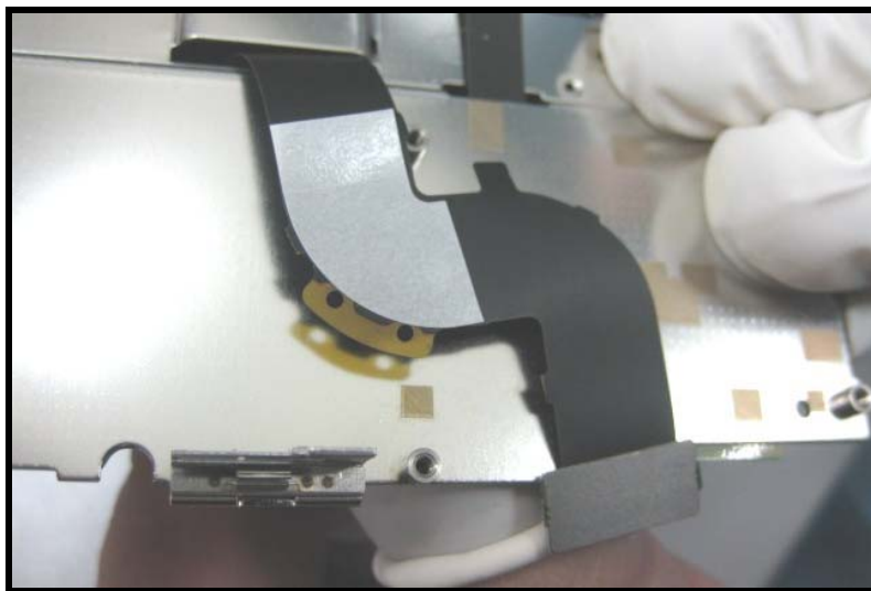
Figure 92. Pulling dynamic flex through slider
