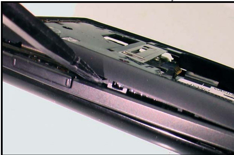
Figure 13. Releasing locking tab near volume key
