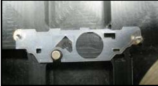
Figure 119. Audio gasket alignment
