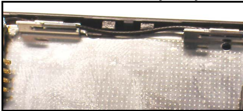
Figure 137. RF coax wire alignment
