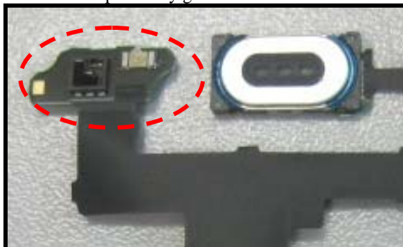
Figure 72. Placing proximity grommet
