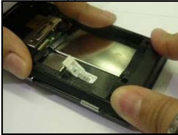
Figure 148. Assembly of rear housing
