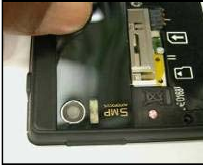
Figure 157. Placing camera/flash cover
