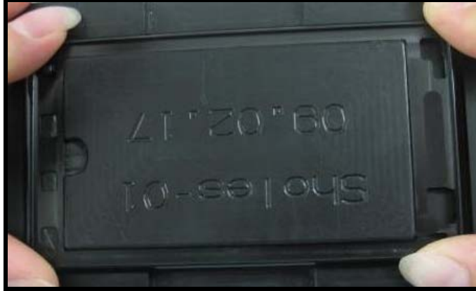
Figure 63. Pressing slider housing over LCD gasket
