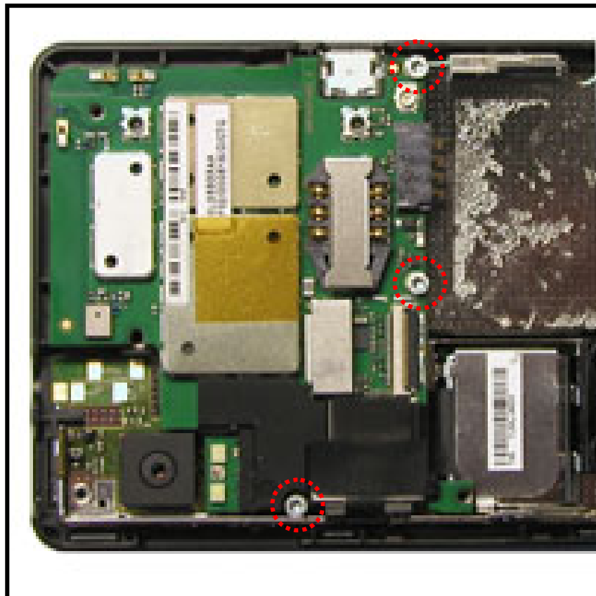
Figure 17. Removing PCB screws (3 points)
