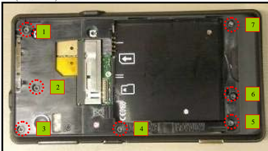
Figure 150. Installing rear housing screws (7 points)
