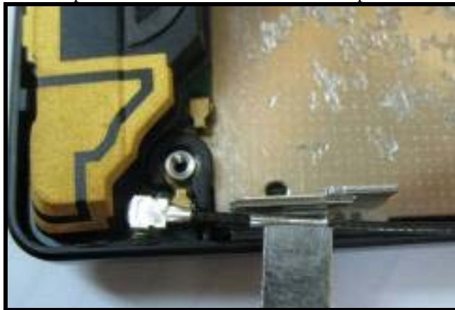
Figure 134. Clamping RF coax wire
