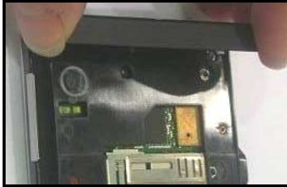
Figure 151. Attaching antenna cap
