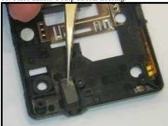
Figure 141. Placing adhesive for headset jack
