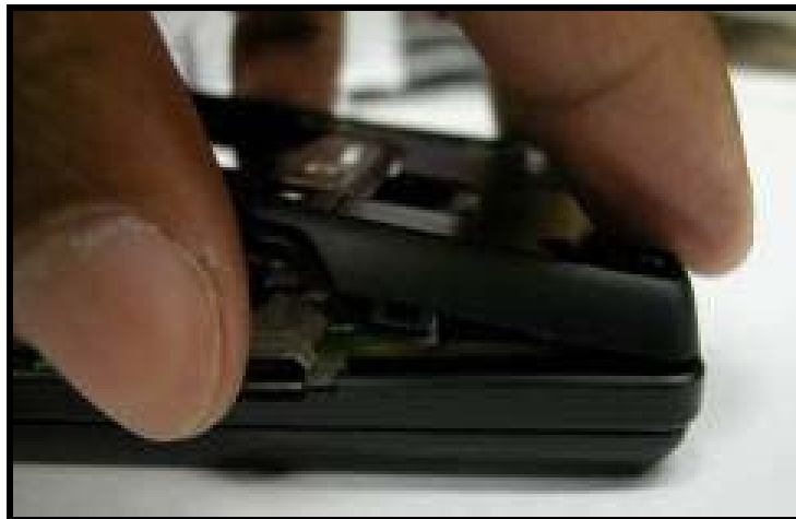
Figure 146. Rear housing assembly
