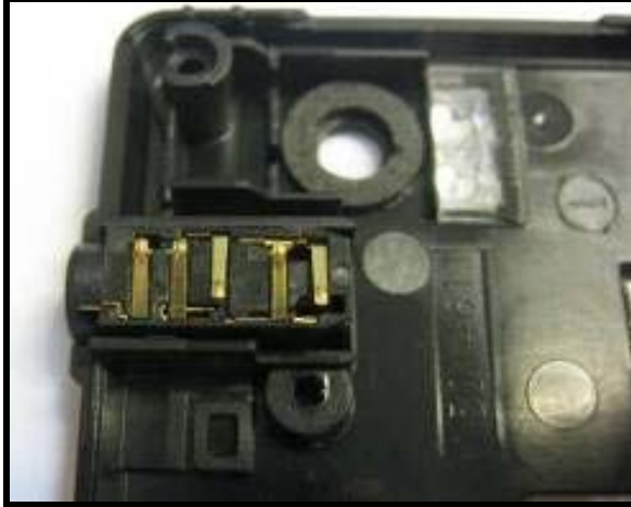
Figure 142. Placing headset jack
