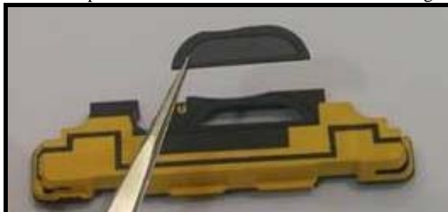
Figure 126. Placing loudspeaker screen
