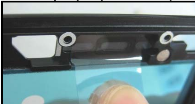
Figure 67. Removing earpiece speaker port adhesive backing
