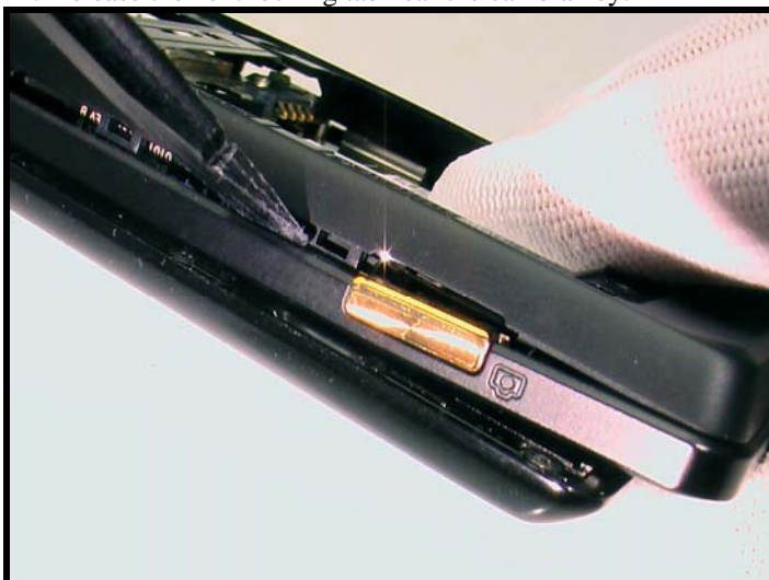
Figure 14. Releasing locking tab near camera key
