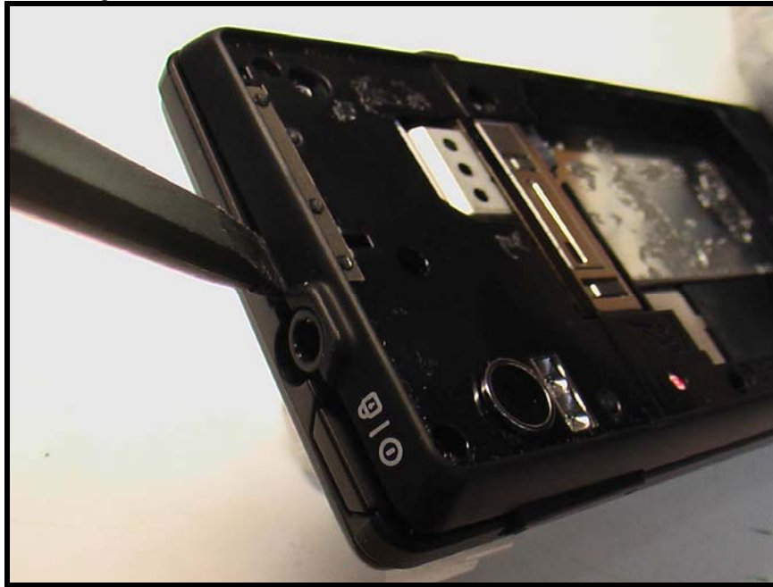
Figure 10. Releasing locking tab near headset jack
