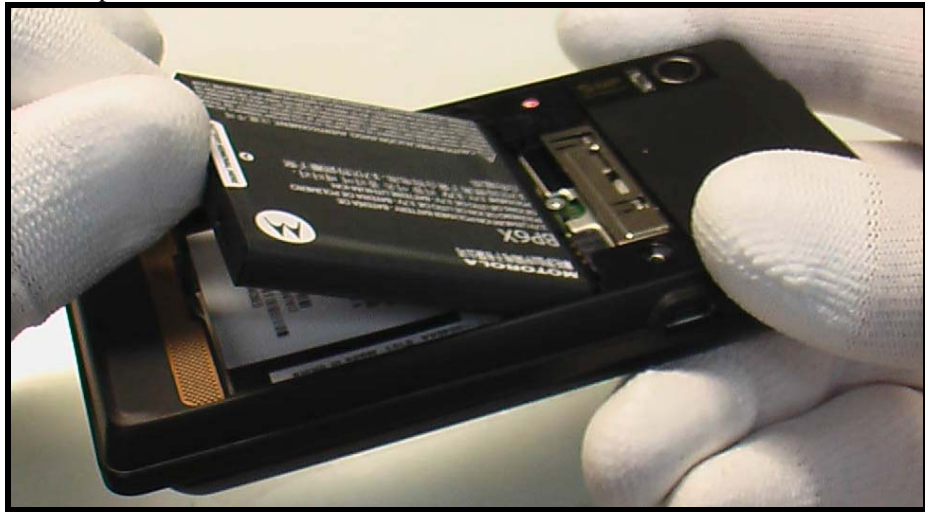
Figure 3. Removing the battery
