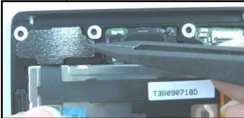
Figure 78. Placing water ingress over ITO connector
