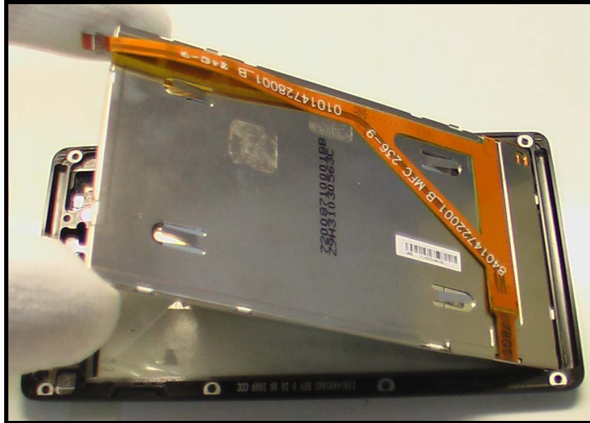
Figure 49. Lifting the display module
