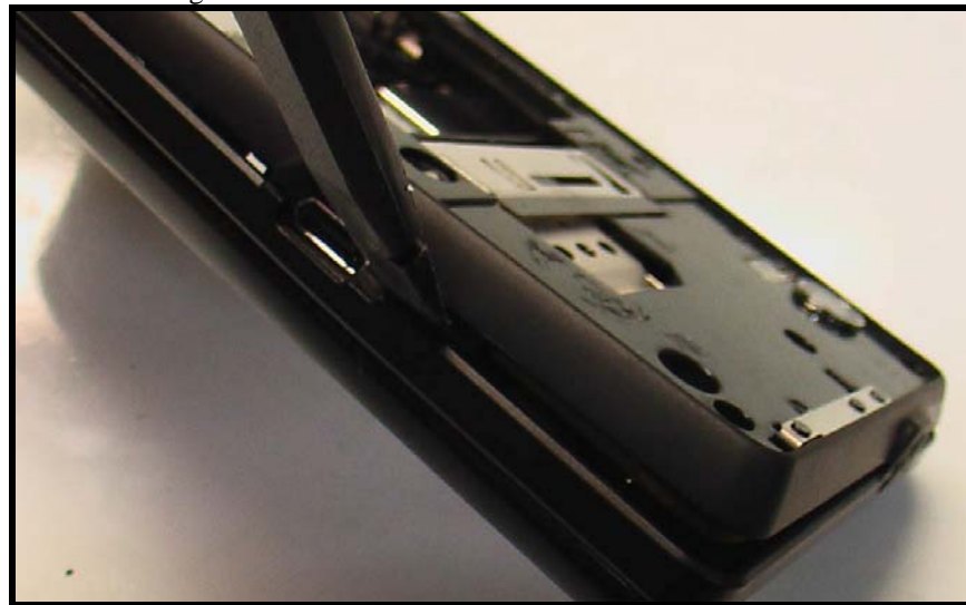
Figure 11. Releasing locking tab near USB connector
