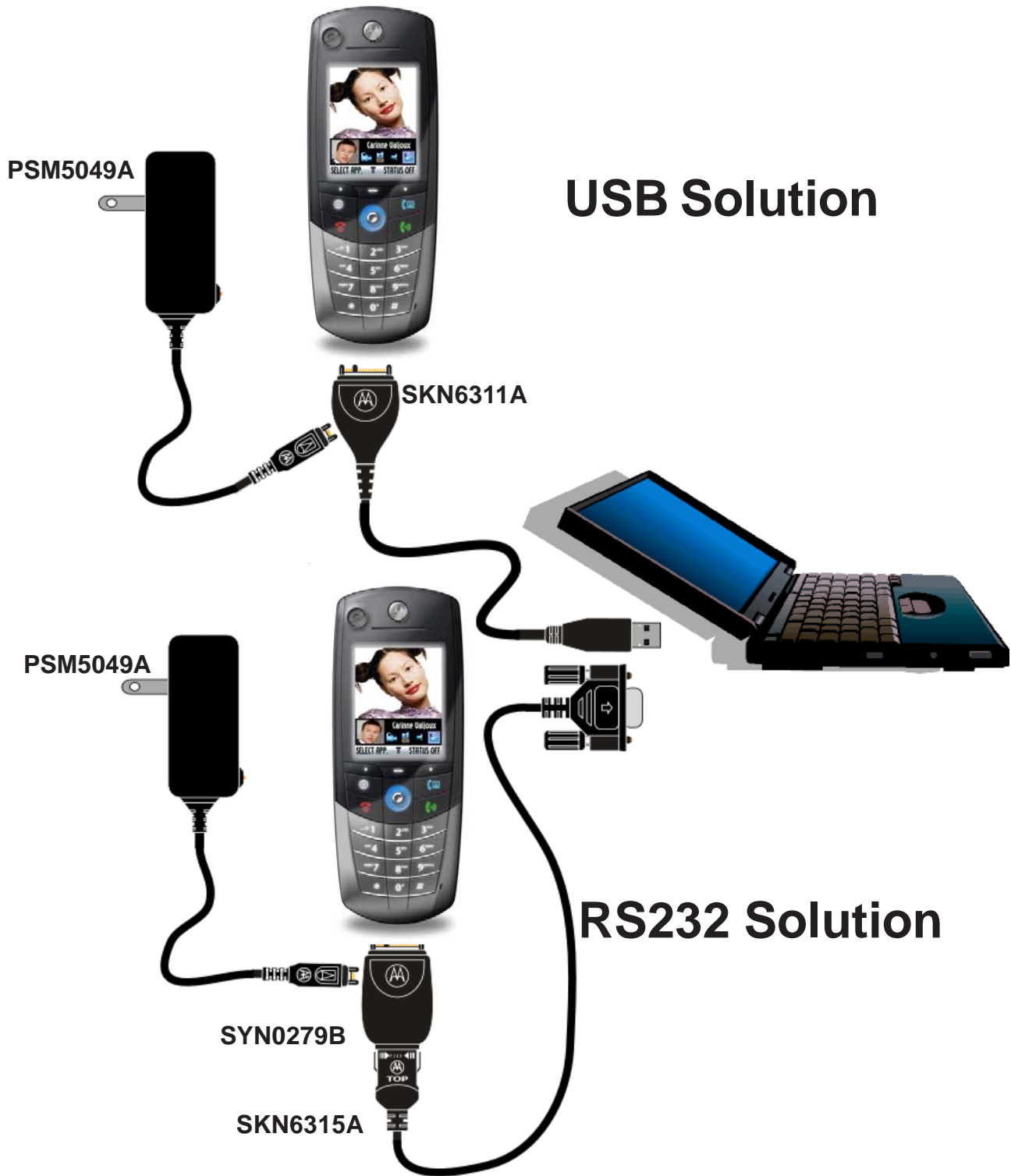
Figure 1-1. PST Hardware Configuration
