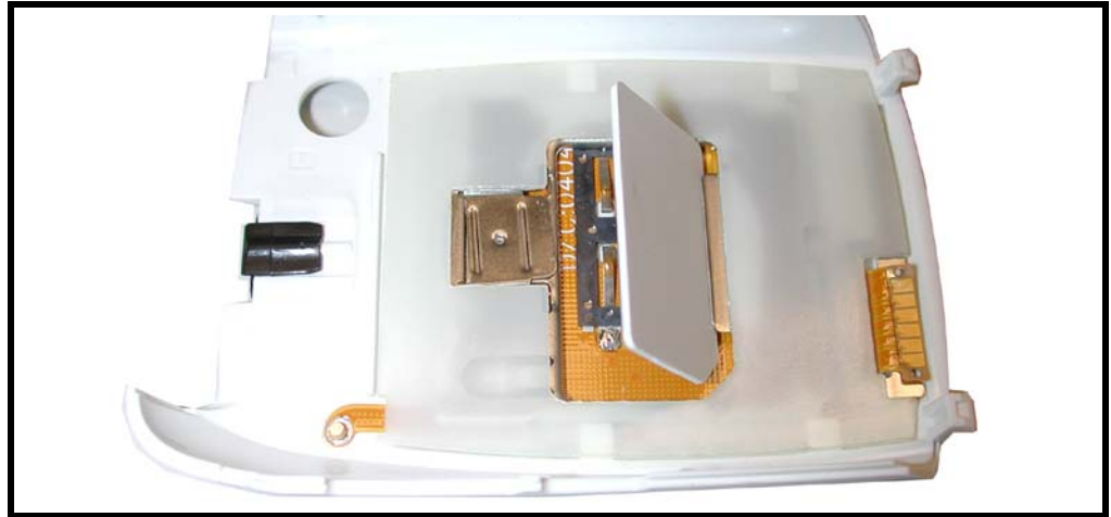
Figure 10. Removing the RUIM
