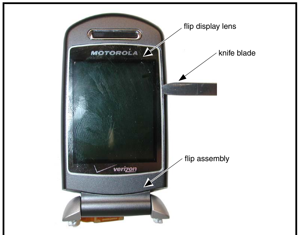
Figure 20. Removing the Flip Display Lens
