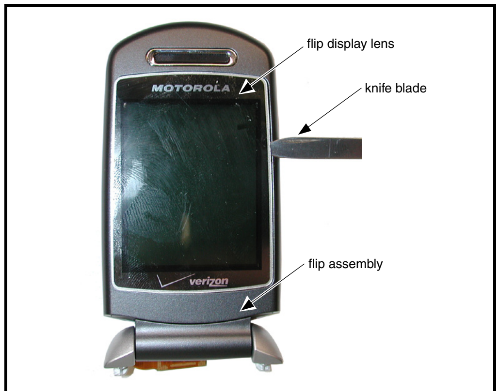
Figure 20. Removing the Flip Display Lens
