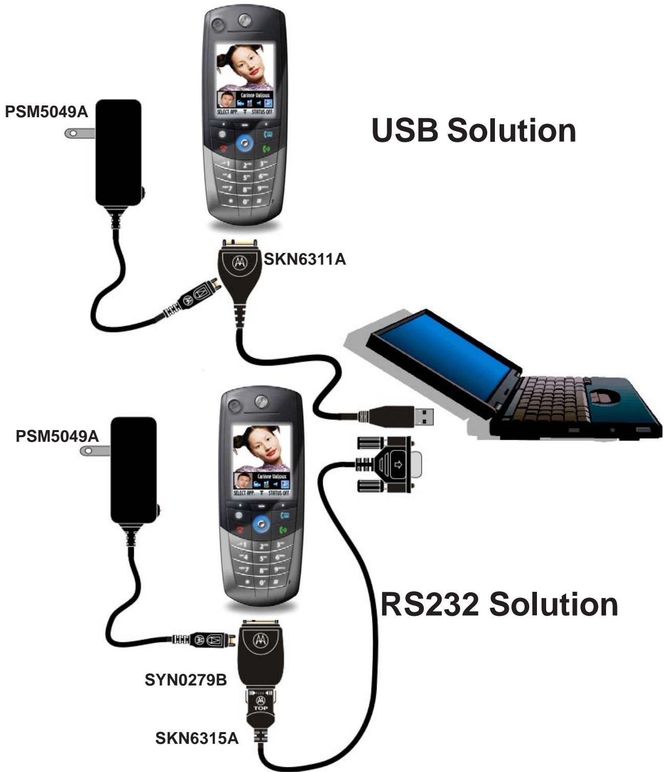
Figure 1. PST Hardware Configuration
