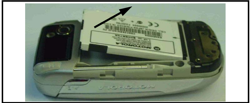
Figure 2. Removing the battery
