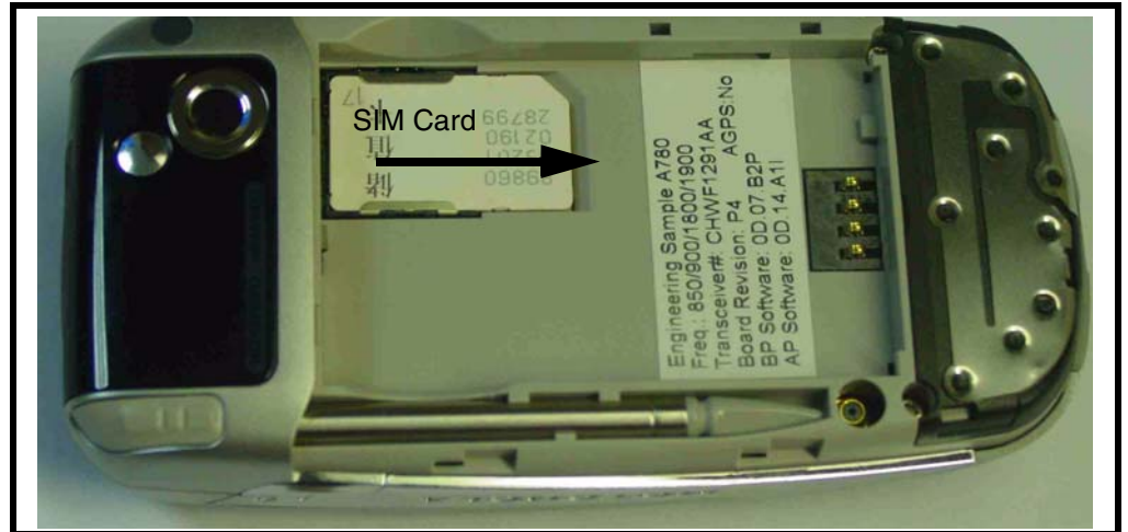
Figure 3. Removing the SIM
