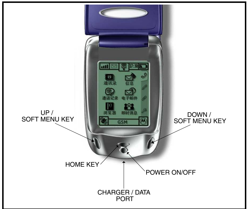
Figure 1. A388c Telephone Controls, Indicators, and I/O
