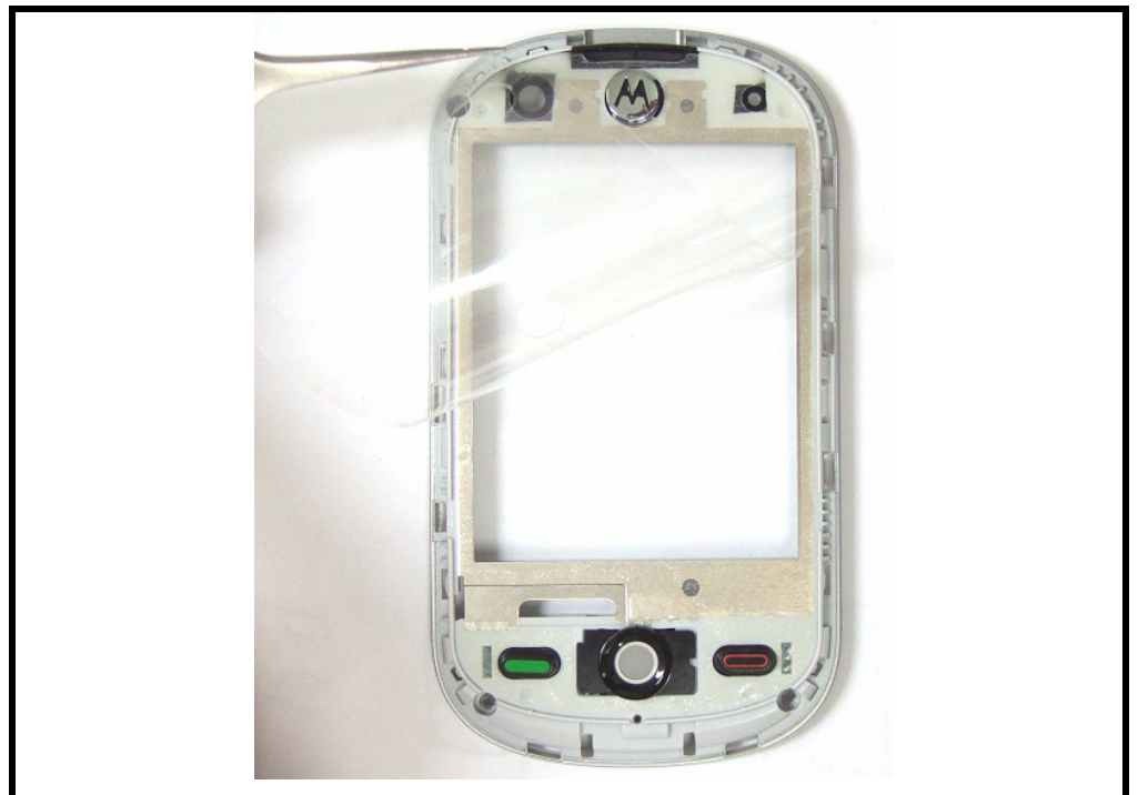
Figure 36. Removing the Liner
