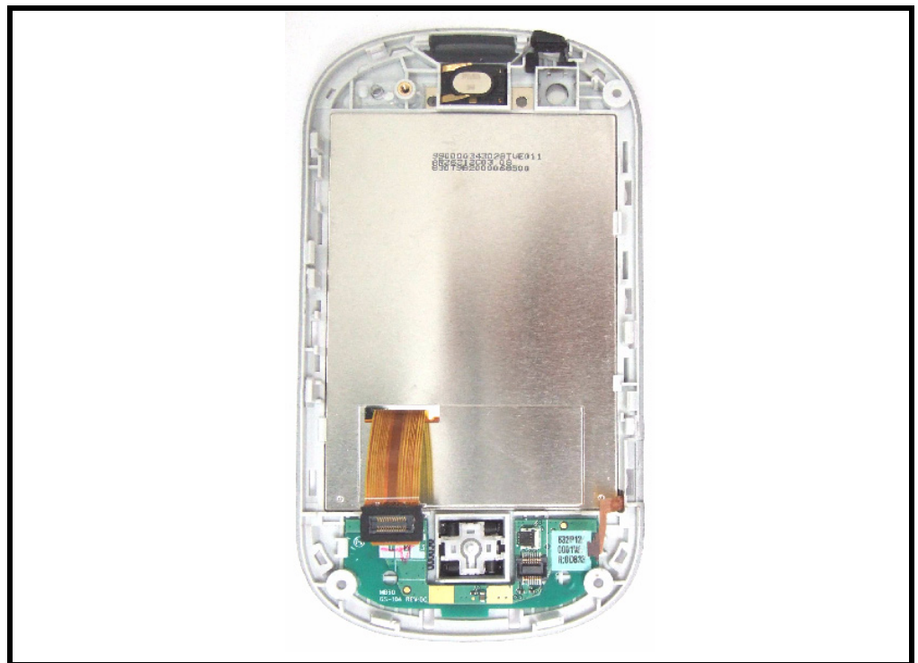
Figure 40. Inserting the LCM
