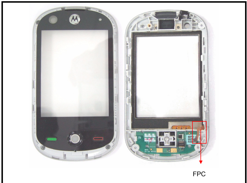
Figure 38. Inserting the FPC
