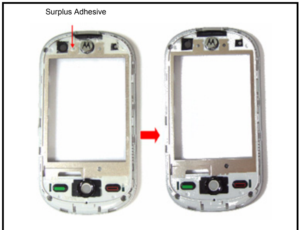
Figure 34. Removing the Surplus Adhesive
