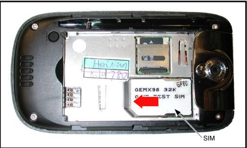
Figure 8. Removing the SIM
