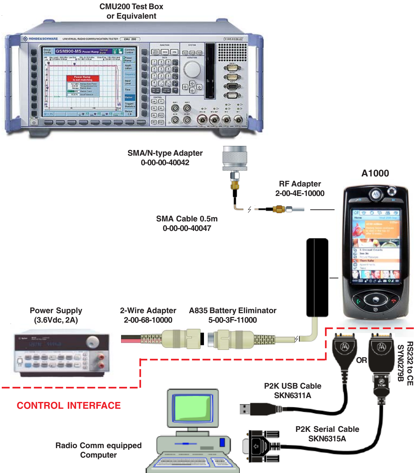
Figure 2-5. A1000 Manual Test Hardware Configuration
